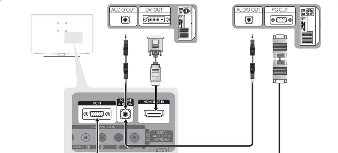
The diagram shows a TV's rear panel with PC audio ports. Two PC configurations are shown: one with **AUDIO OUT** and **DVI OUT**, and another with **AUDIO OUT** and **PC OUT**. Cables connect the TV's **PC IN** (D-sub), **PC AUDIO IN** (3.5mm), and **HDMI (D) IN** (HDMI) ports to the corresponding ports on the PC.
